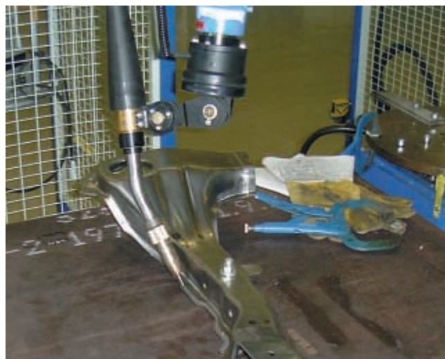
Interior from the robot cell in Göteborg where a front suspension part is test welded with OK Tubrod 14.11 Ø 1.4 mm.
