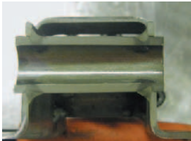
Example of the very good penetration also at high welding speeds, in this case 27 mm/sec.
